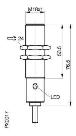
Inductive Sensors BES 516-538-BO-H-M18x1 x 76.5 normally-open Sn=5mm shielded
